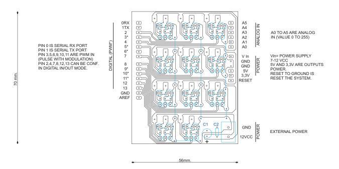
R1=1000 OHM 1/4 WATT 5% R2=4700 OHM 1/4 WATT 5% R3=10000 OHM 1/4 WATT 5% C1=100 microF 25 V elettrolitico C2=100 nanoF multistrato LED1= DIODO LED 3mm. rosso T1= NPN BC547
