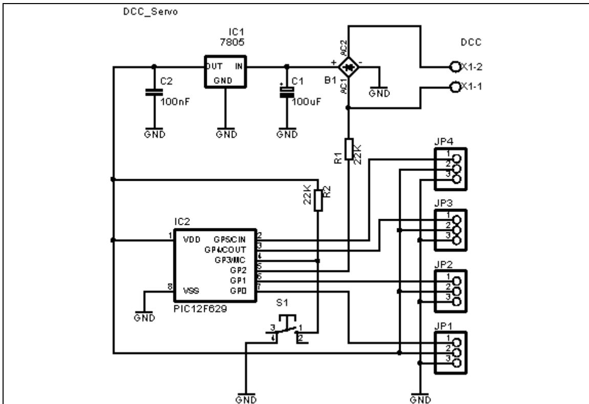
To control a servo we will have to apply a pulse of specific duration and frequency, the servo have three wires, two for feeding Vcc and Gnd and another wire to apply the control pulses that will cause that the servo moves to the position indicated by the width of the pulse (pin 1 of each servo connector)
